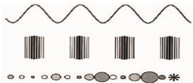
Fig. 2: Compression and expansion cycle of ultrasound [9, 14, and 15]
